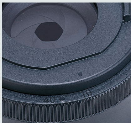
Field diaphragm with position guide markings
